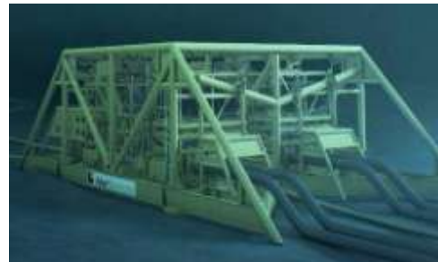
Åsgard subsea compression system
